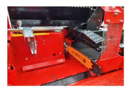
The traditional blade is suitable for handling large quantities, whereas the Perfect Split blade ensures a top-quality finish. The ergonomic new interface enables one-handed operation, where sawing is done by holding down the joystick button, and the clear interface makes working intuitive.
